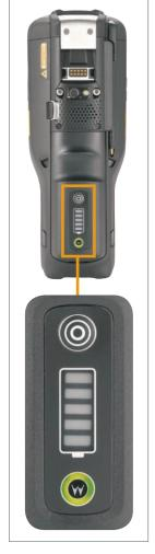
A patent-pending easy-to-read intelligent graphical display right on the battery itself presents the state of charge as well as the state of battery health — and the display is always available. When the battery is in a charger, the display is automatically activated. When the battery is standalone or installed in the MC9500-K, a quick press of the status button activates the display.\*
